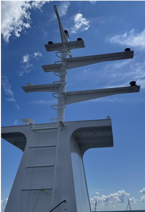
7086 – PH Mast w/Navigation Lights Being Installed
