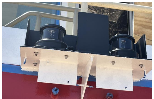
7091 – Side Navigation Lights on PH Structure
