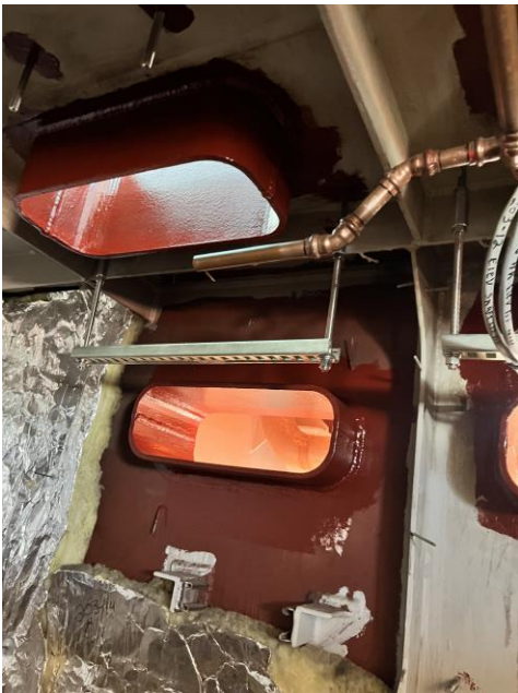
6924 – Bulkhead Penetration into 02 Deck Restroom with Primer Paint
