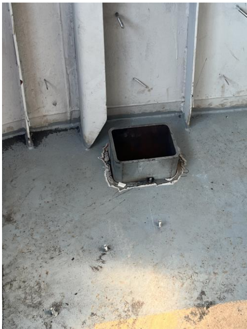
6815 – Penetration Collar from Electronics Room to Pilot House
