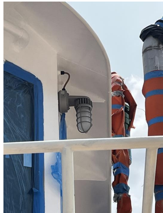
6768 – Lighting Installed at Pilot House
