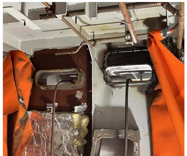
6821 – Bulkhead Penetrations from 02 Crew Restroom to Outside
