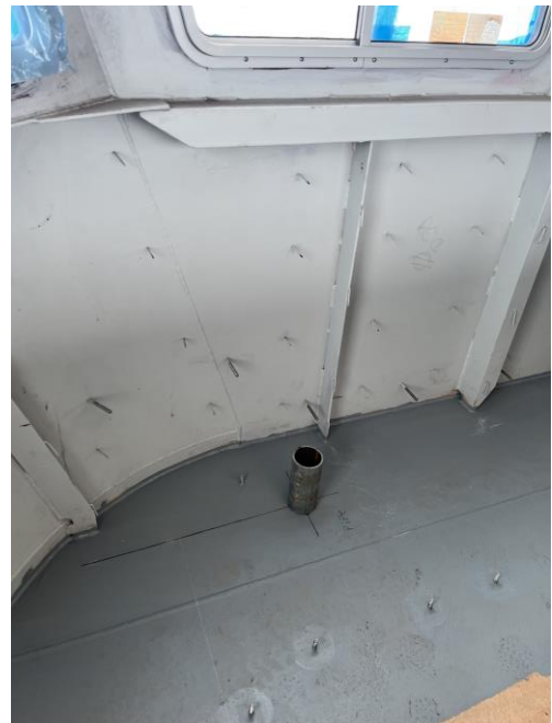
6807 – Electrical Penetration into Pilot House
