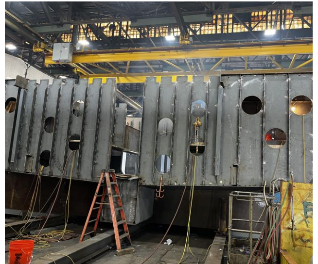
2761 – One section of Main Deck placed on Module 4
