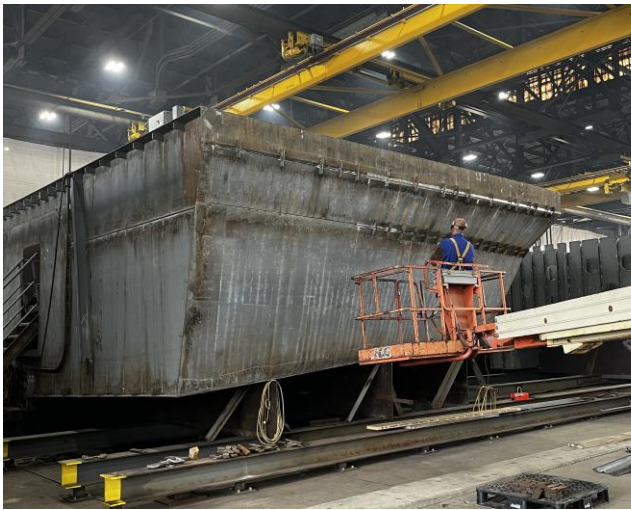
Pic 2683 – Module 2, welding hull flare near deck level
