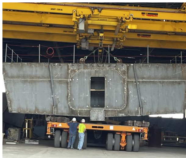
2889 – Module 2 being loaded for transport to paint shed
