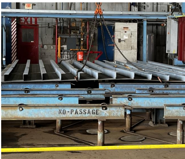
2739 – Main Deck section ready to be flipped and placed on Module 4
