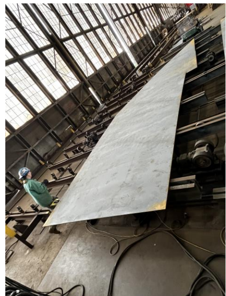
2764 – Bottom Plate cut for Module 1
