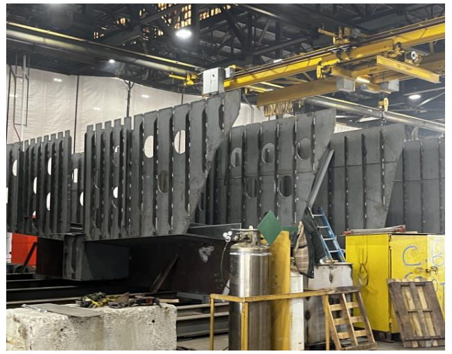
Pic 2684 – Module 4 bulkheads being installed
