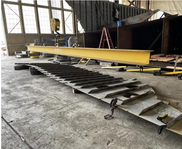
2929 – Bulkhead for Module 1 ready to be lifted into place
