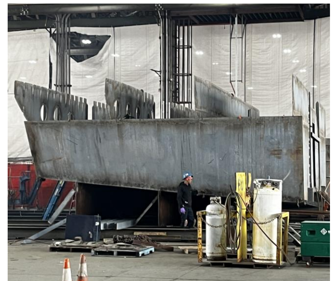
2693 – Hull side plating on Module 4
