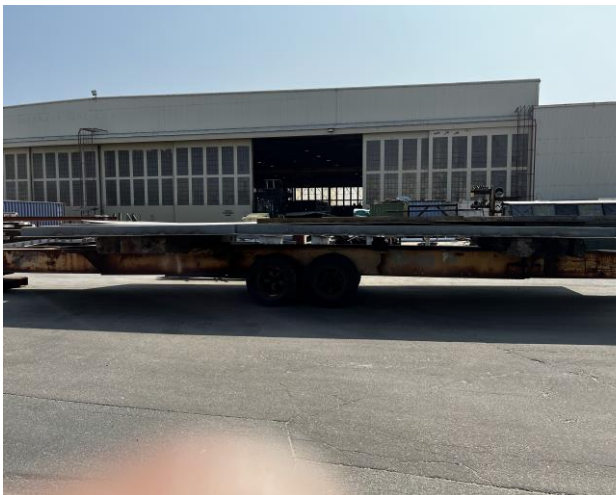
2941 – Trailer (called the Turtle) moving bottom shell plating for Module 5 from the cutting area to the fabrication area
