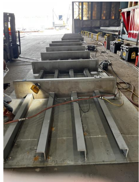
2738 – Assembled Main Deck section for Module 4
