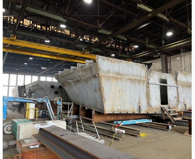
2730 – Starting Hull flare at deck on Module 4
