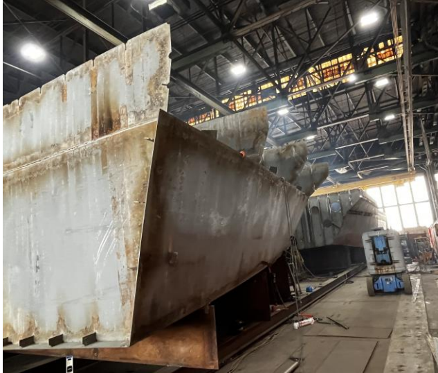
2695 – Hull side plating for Module 4
