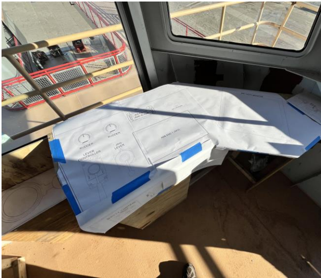
5827– Pilot House Console Mock-Up w/Location of Controls Laid Out
