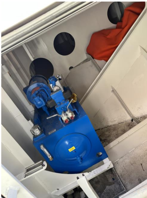
6061 – Jastram Hydraulic Unit for Steering System in Lazarette
