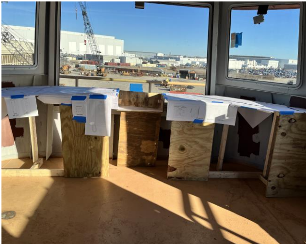
5823 – Pilot House Console Mock-Up w/Location of Controls Laid Out
