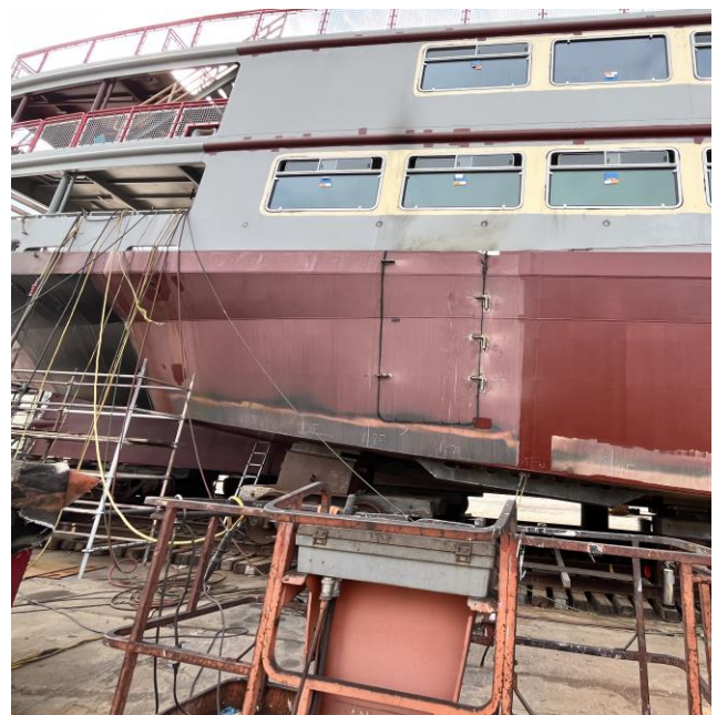
6025 - Hull Access Hole Cut for Loading Equipment in Switchboard Room
