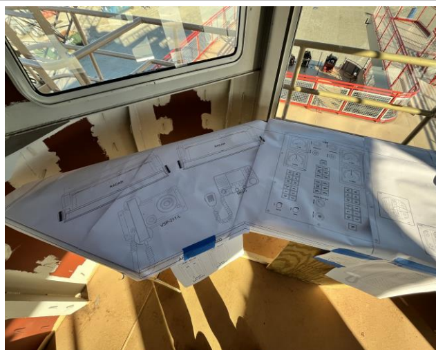
5825 – Pilot House Console Mock-Up w/Location of Controls Laid Out
