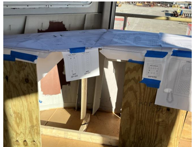
5824 – Pilot House Console Mock-Up w/Location of Controls Laid Out
