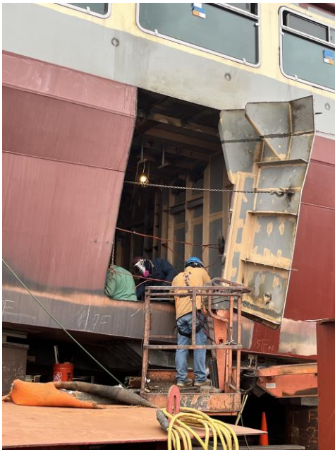
6028 - Hull Access Hole Cut for Loading Equipment in Switchboard Room
