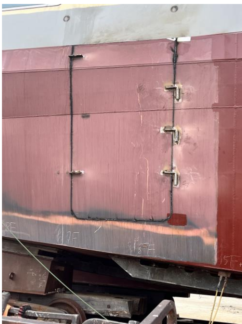
6024 – Hull Access Hole Cut for Loading Equipment in Switchboard Room
