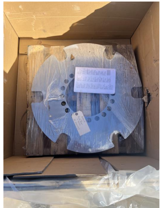
5933 – Brake Rotor for the Torsional Coupling
