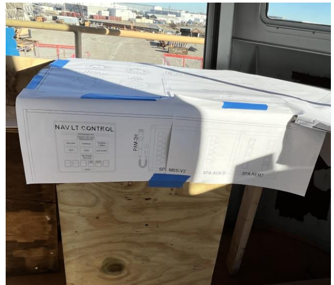
5828 – Pilot House Console Mock-Up w/Location of Controls Laid Out
