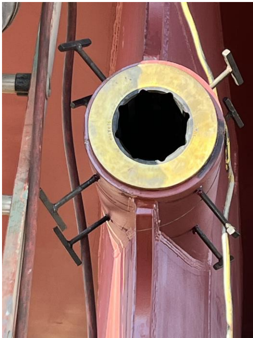
5978 – Shaft Cutlass Bearing on Stern Tube
