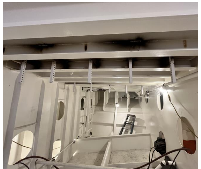
5977 – Access Hatch Handle, Downcomer Lighting Supports and Piping Valves in a Void Space
