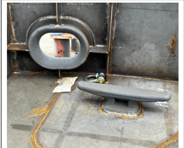
4134 – Fully Welded in Keel (Cleat) With Line Chock in Bulwark
