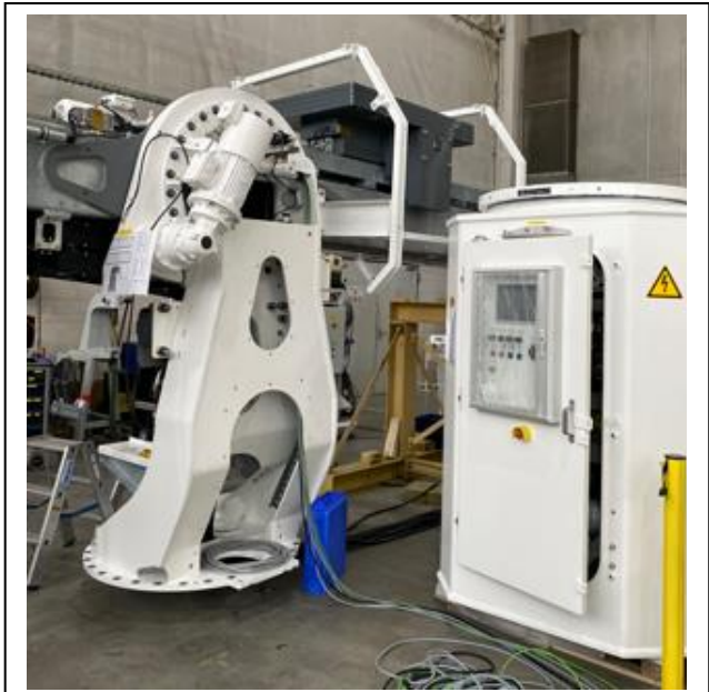
Charger 7 – Charger Tower Base with Ring Partially Attached. Ready for Next Section
