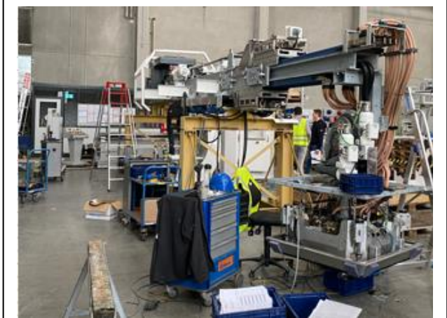
Charger 6 - Adding Charger Plug to Telescoping Arm with Wiring Going In
