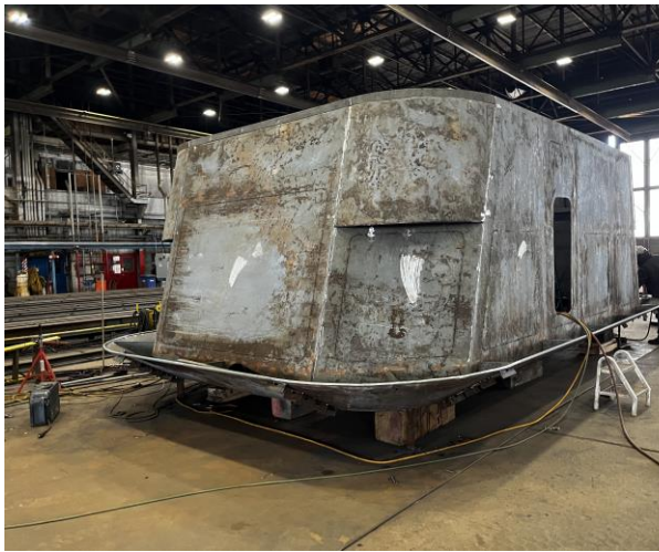
3890 – Pilot House being constructed upside down
