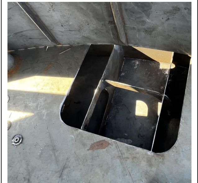
4061 – Kevel Plate Opening with Stiffener Added
