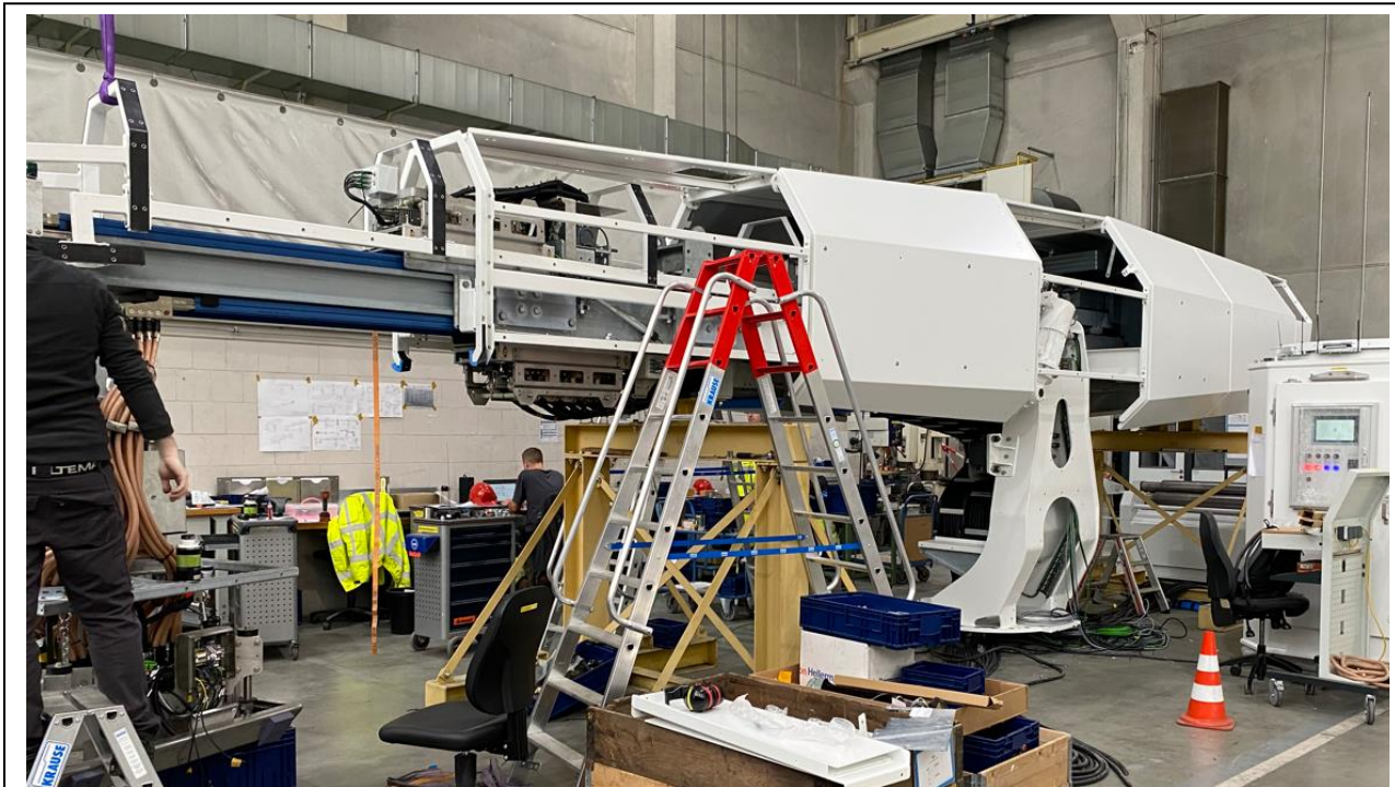
Charger 1 – Charger Arm with Additional Housing In Place
