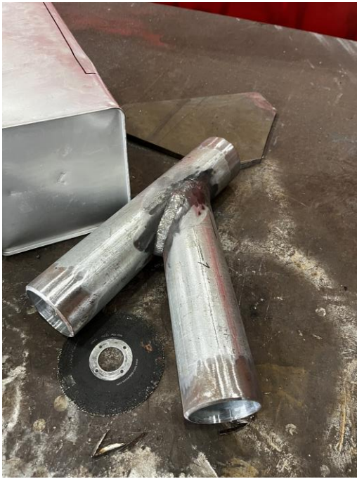
3999 – Deck Drain Piping Section
