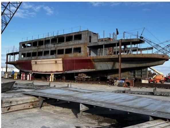
3737 – View of Starboard Side with Vessel being Readied to Receive Module 9 Deck Sections (in foreground)
