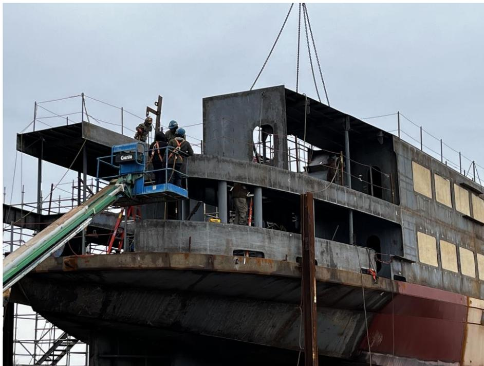
3830 - Setting Module 9 deck plating (02 Deck) on stern of vessel
