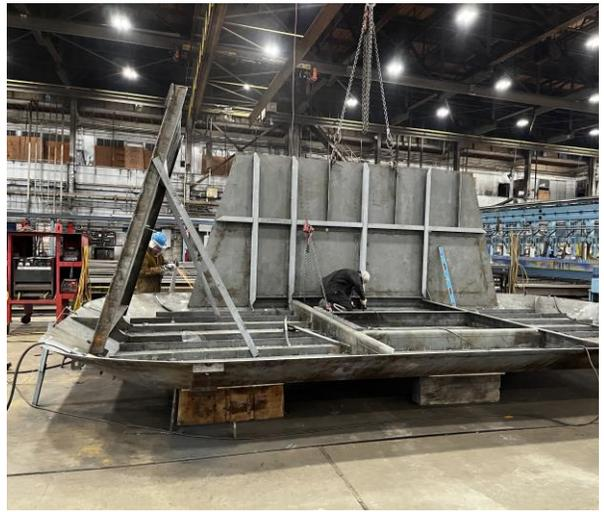
3832 - Placing Pilot House Bulkheads – house is being constructed upside down.
