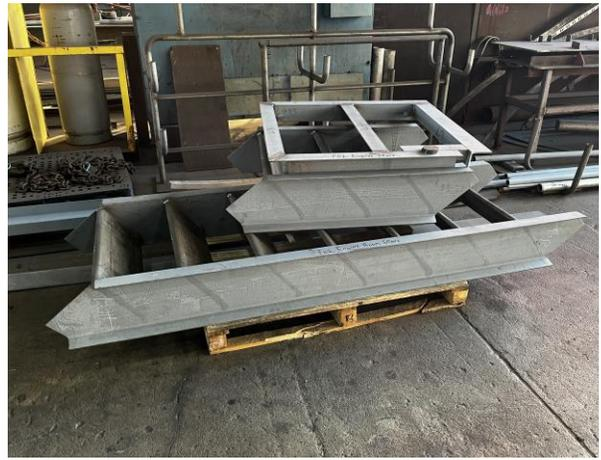
3601 – Stair Sections Fabricated for the Vessel
