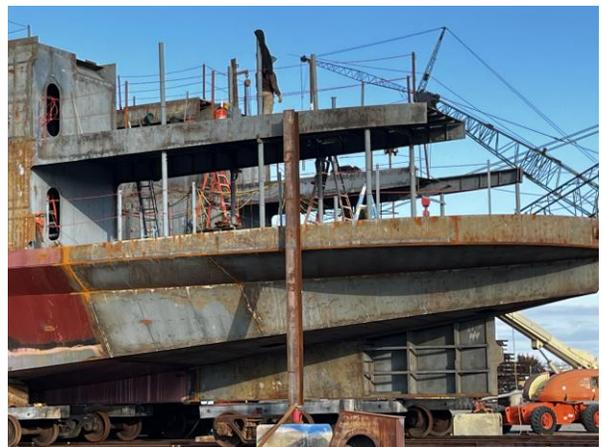
3739 - View of Starboard Side with Vessel being Readied to Receive Module 9 Deck Sections
