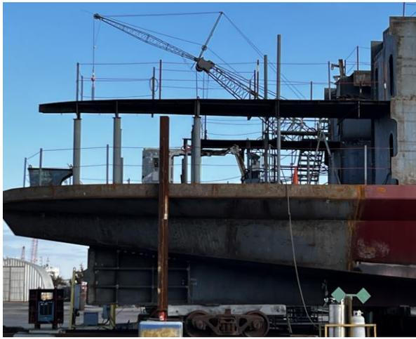
3740 - View of Port Side with Vessel being Readied to Receive Module 9 Deck Sections
