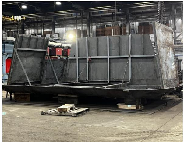
3834 - Placing Pilot House Bulkheads – house is being constructed upside down.
