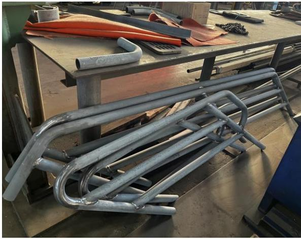
3600 – Handrail Sections Fabricated for the Vessel
