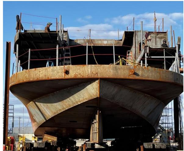
3736 - Installing Stanchions on Module 6 in Preparation of Installing Module 9 (02 Deck outside decking)
