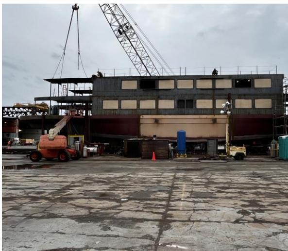
3765 – Port Side, setting Module 9 Decking in Place (02 outside decking)
