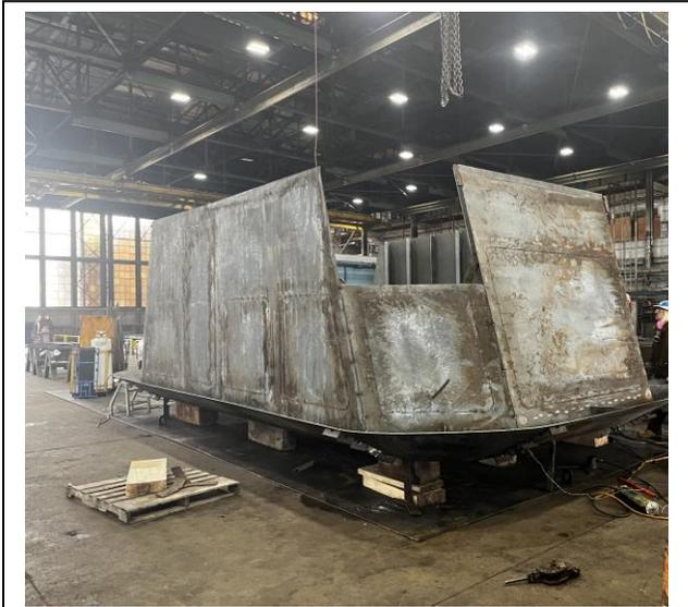
3838 - Placing Pilot House Bulkheads – house is being constructed upside down.
