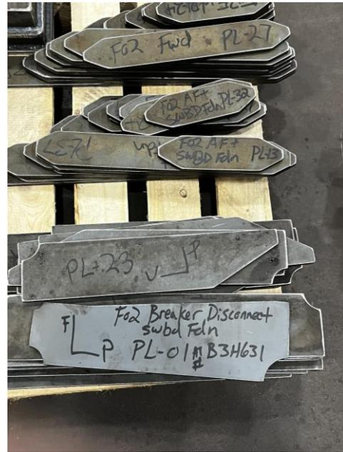
3770 – Various Plates for Equipment Foundations and Stiffeners
