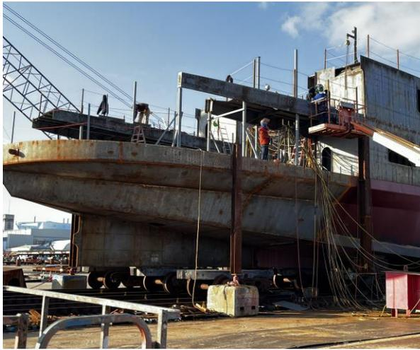
3734 – Installing Sections of Module 6 (bow end) to make up 01 Outside Decking
