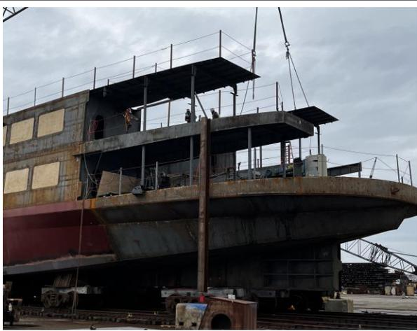
3768 – Starboard Side, setting Module 9 Decking in Place (02 outside decking)
