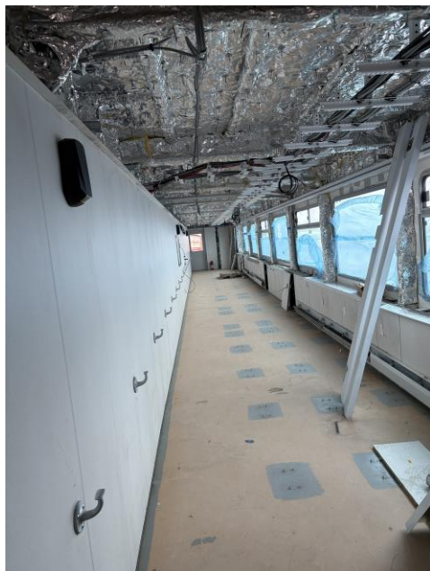
9309 – Handrail Support Being Installed in 01 Deck Port Cabin
