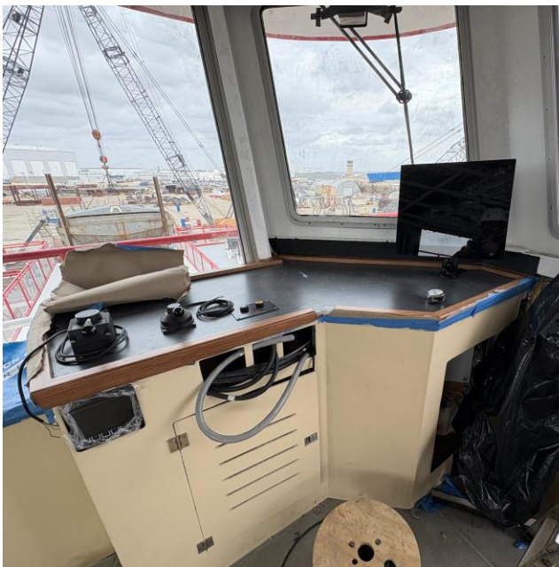
9310 – Stern PH Console w/Steering Controls Being Installed
