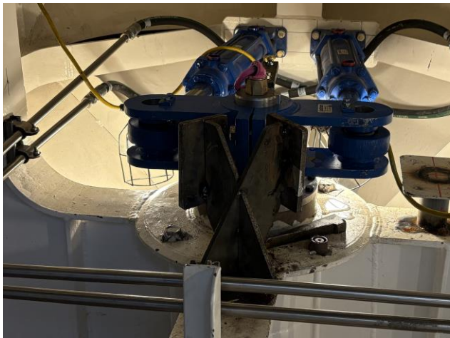
9352 – Hydraulic Steering Unit in Lazarette
