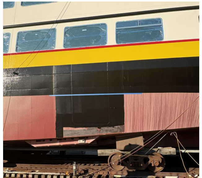
9126 – Painting Hull Where Access Opening was for Load Out
