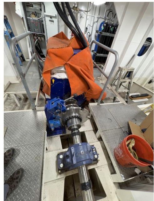
9085 – Torsional Coupling Bearing W/Manual Brake System in Place
