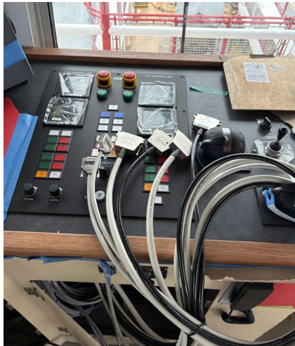
9446 – Wiring for Controls on PH Console
