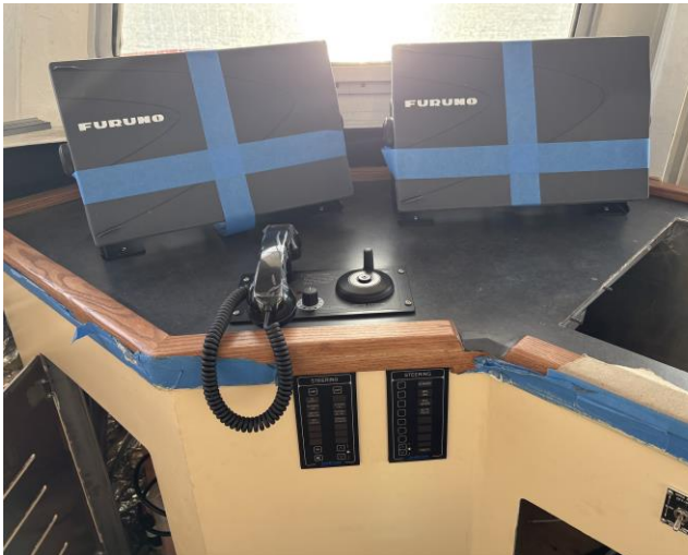
9346 – Radars, Phone & Steering System Warning Panels in PH Console
