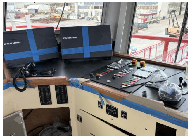
9311 – Stern PH Console w/Throttle Controls, Propulsion Panel & Radars Being Installed
