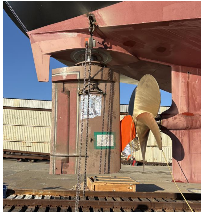
9027 – Installing Bow Rudder
