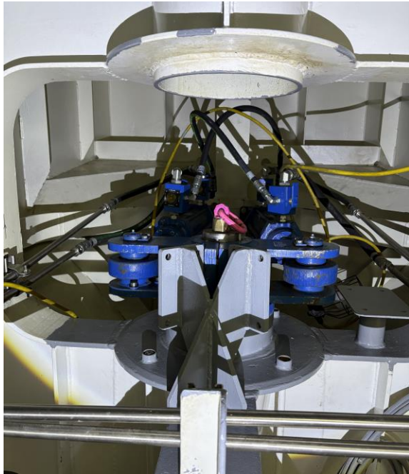
9487 – Hydraulic Steering Unit in Lazarette-Painted
