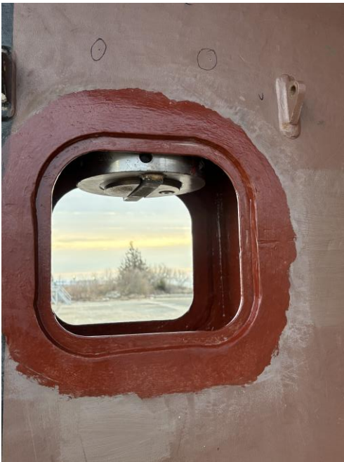
9498 – Temp. Access for Rudder Stock Assembly
